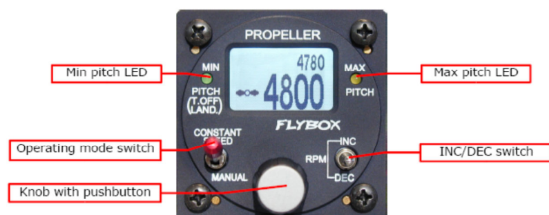
Fig. 11 Electronic constant speed instrument
